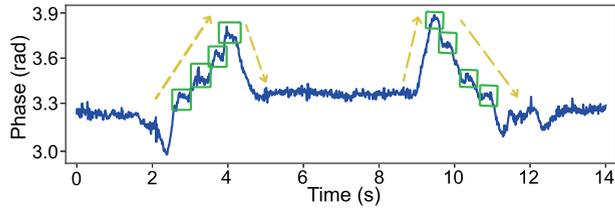
Fig. 9. Phase of multipath signals caused by a person walking by.
