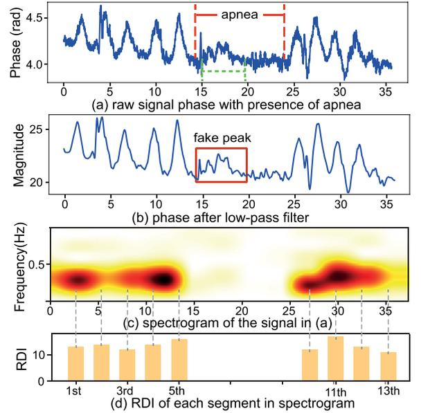
Fig. 14. Raw phase, phase after matched filter, spectrogram, and RDIs for the respiration signal with apnea.
