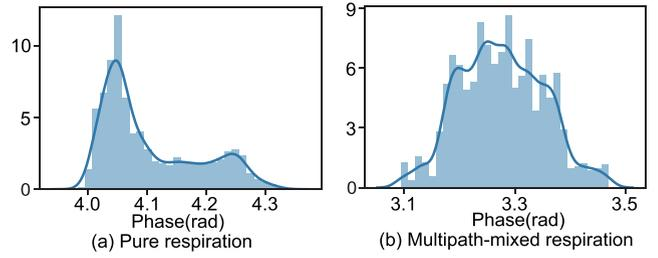
Fig. 16. Distributions of the signal phase for (a) the pure respiration signal and (b) respiration signal mixed with the multipath signals.
