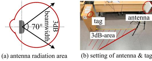
Fig. 5. Illustration of RFID antenna radiation range and 3 dB beamwidth.
