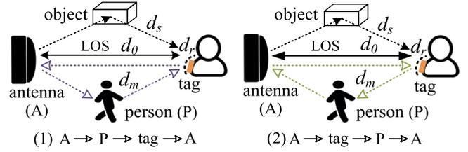
Fig. 3. Propagation path of multipath signals from moving person.
