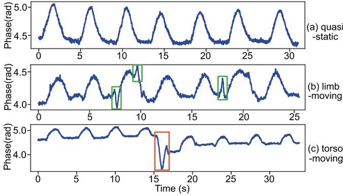
Fig. 13. Signal phase for respiration under different movement status.
