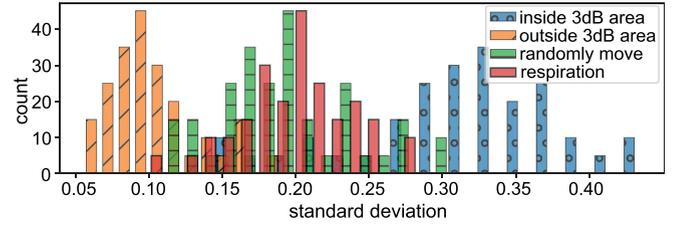
Fig. 7. Distribution of standard deviation of the signal phase with moving people moving in different areas.
