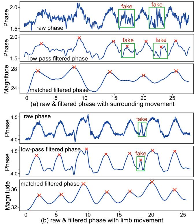
Fig. 18. Raw and filtered phase mixed with the multipath signals from (a) the ambient movement of surrounding people and (b) the limb movement of the monitored person.
