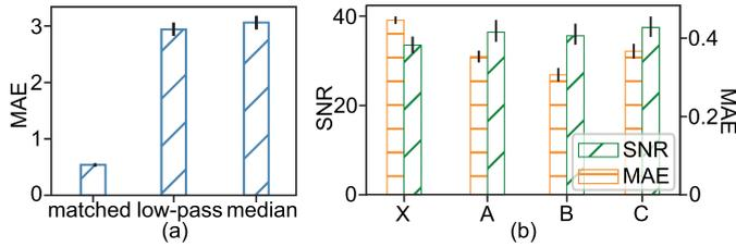
Fig. 20. Effect of matched filter: (a) MAE for respiration rate estimation with matched filter, low-pass filter, and median filter (b) SNR and MAE of using different respiration templates to make matched filter.
