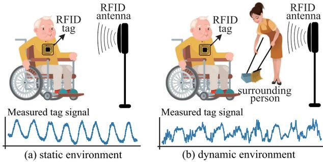
Fig. 1. Respiration monitoring in the static and dynamic environments. The signal in the dynamic environment suffers from many noises compared with that in the static environment.
