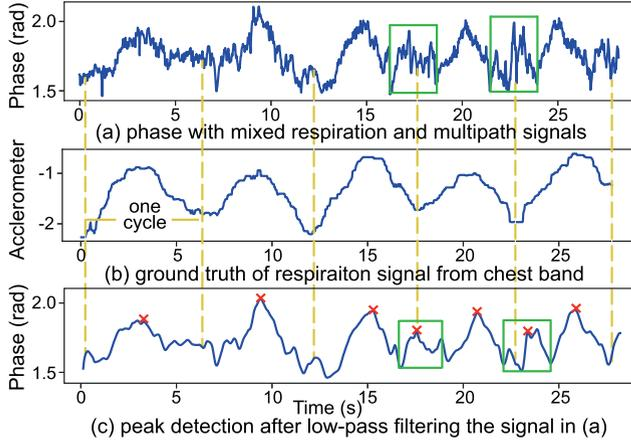
Fig. 10. Multipath mixed respiration signal, ground truth respiration signal, and peak detection result.
