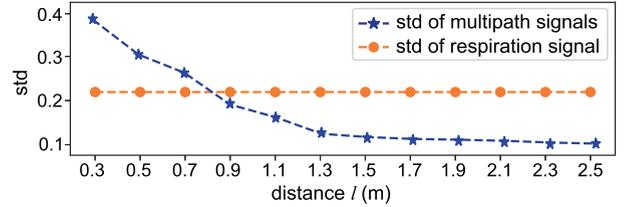
Fig. 8. Standard deviation of signal phase for different distances  $l$ .
