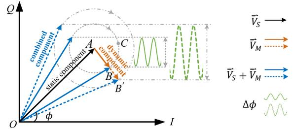
Fig. 4. Effect of dynamic multipath signals on the signal phase.
