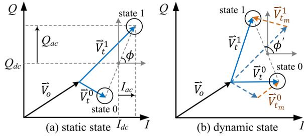
Fig. 2. Demodulated voltage of the tag signal received by RFID reader.
